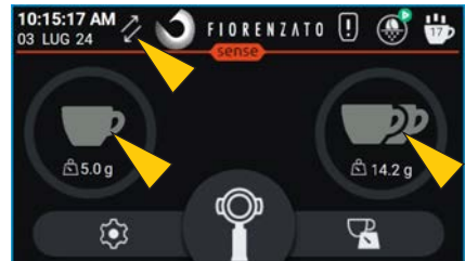
HOME screen with “SENSE” system active and communicating with weighing group
